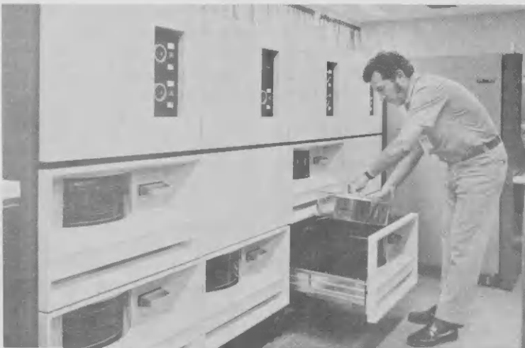
Part of the new equipment includes this Disk Storage Unit, where six disk-packs are kept.
